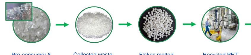
Pre-consumer & Post-consumer plastic collected & sent to a recycler Collected waste sorted, washed, dried & chopped into flakes Flakes melted, extruded and pelletized
